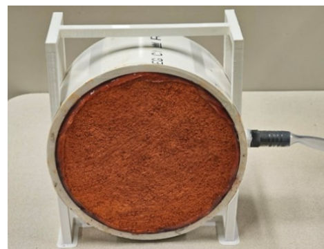
Figure 6. Photo of GWF of ceramic filter showing the stand, the handle (on top), and the exit tube which carries the treated water to the filtered water container.
