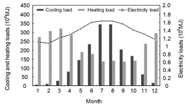
**Figure 1.** Schematic diagram of the hot, cold, and power load of a hotel in Shanghai.
