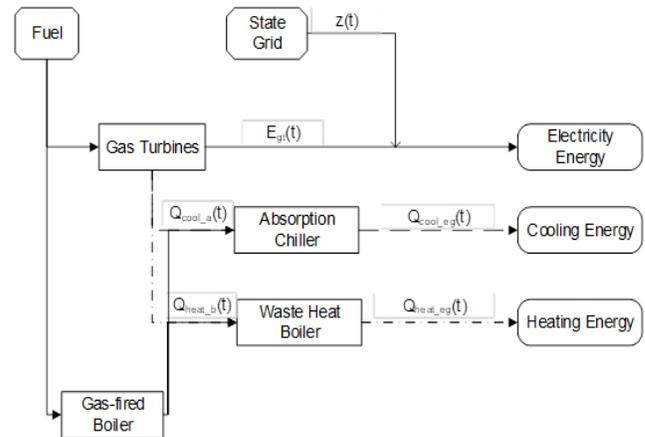
Figure 5. The structure and components of the CCHP system.
