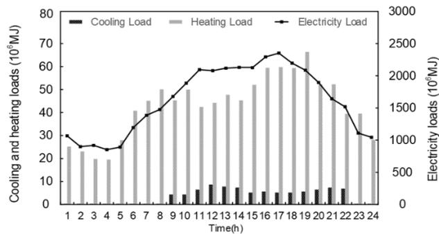
Figure 3. The cold, heat, and electricity load in a typical day of winter.
